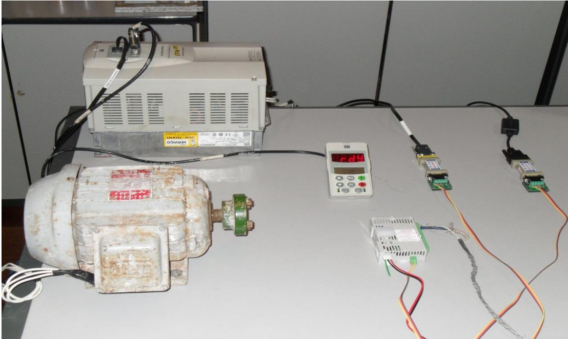
Fig 6.14 – Inversor, motor, IHM, conversores 232/485 e I/O Termopar/485.
